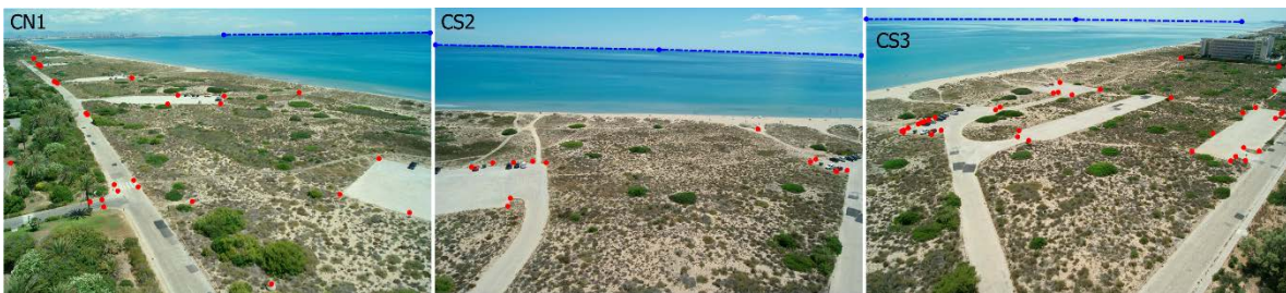
415 416 Fig. 2. Three examples of photos at El Saler beach taken from different camera position on 17 June 2016; the 417 first photo from the north camera (NC) and the other two from the south camera (CS). Distribution of the GPS 418 points in the area is dotted in red and the horizon line is shown in blue. CN1 is an example of where the 419 horizon formulas are obtained by two points, while CS2 and CS3 are obtained by three points. 420
