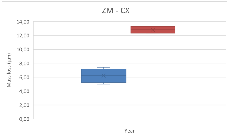
Figure 33: ZM mass 93os for CX corrosivity category boxplot chart
