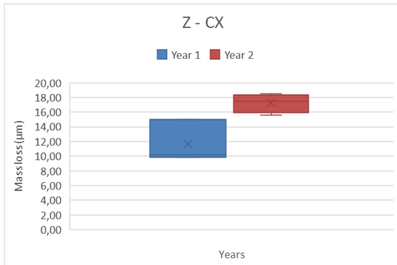
Figure 38: Z mass loss for CX corrosivity category boxplot chart
