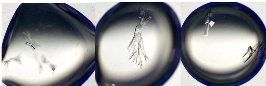
Figure 5. FmtA crystals. FmtA crystals of different morphologies obtained by the hanging drop and vapour diffusion technique. The dimension of the largest crystals is about 0.3 mm. Some of them are small (left), others show branching (centre) and others are large aggregates formed by other smaller crystals (right).
